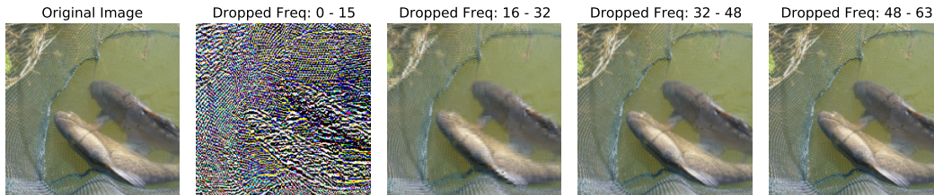
Figure A.18: ImageNet examples where image is reconstructed after dropping (zeroing) certain frequency bands
