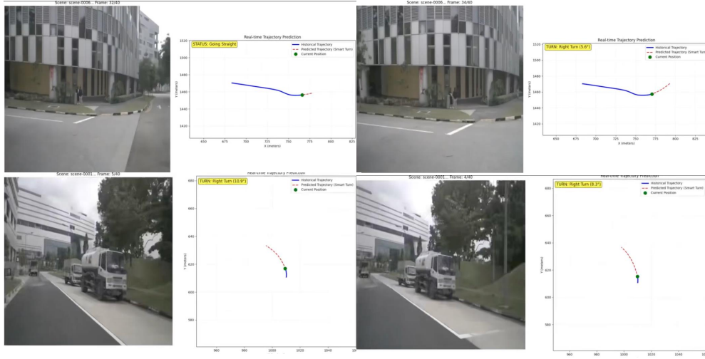
Figure 2: Visualizations of LLM-TrajEcho on nuScene dataset Caesar et al. (2020). The yellow box indicates the predicted motion status: turning angle and direction.
