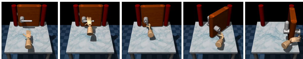
Figure 4: Our learned policies successfully accomplishes manipulation tasks, such as opening a door as shown.
