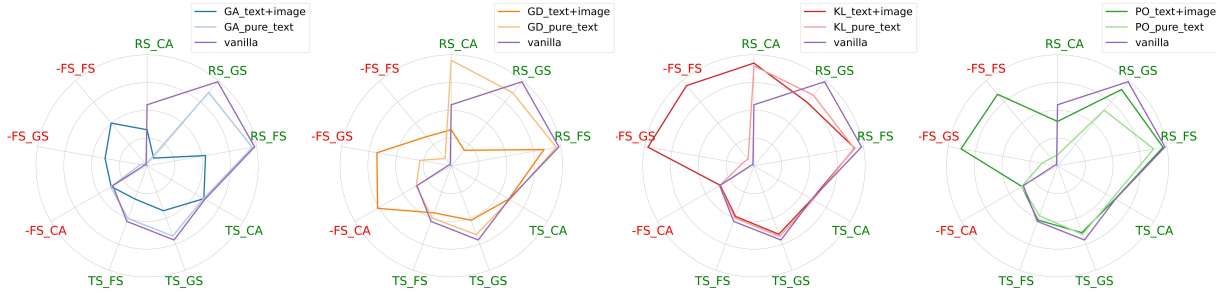
Figure 3: Results of the Unimodal Unlearning. RS, TS, FS represent retain set, test set, and forget set, respectively. CA, GS, FS refer to classification accuracy, generation score, and fact score, respectively.
