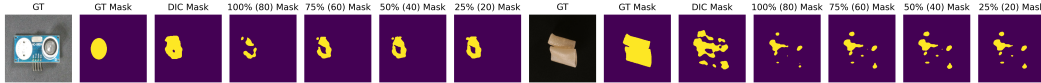
Figure 6: Overview of prediction masks for different levels of maximum static noise levels and the DIC. DIC tends to segment large anomalies more faithfully
