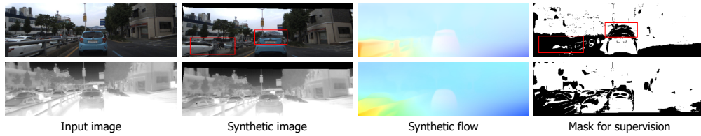
Figure 10: Visualization of the valid mask used for flow supervision on the MS^2 (RGB-T) dataset. Thanks to the photometric consistency checking and the outlier-robust loss, invisible areas and regions affected by severe artifacts are excluded from loss computation.
