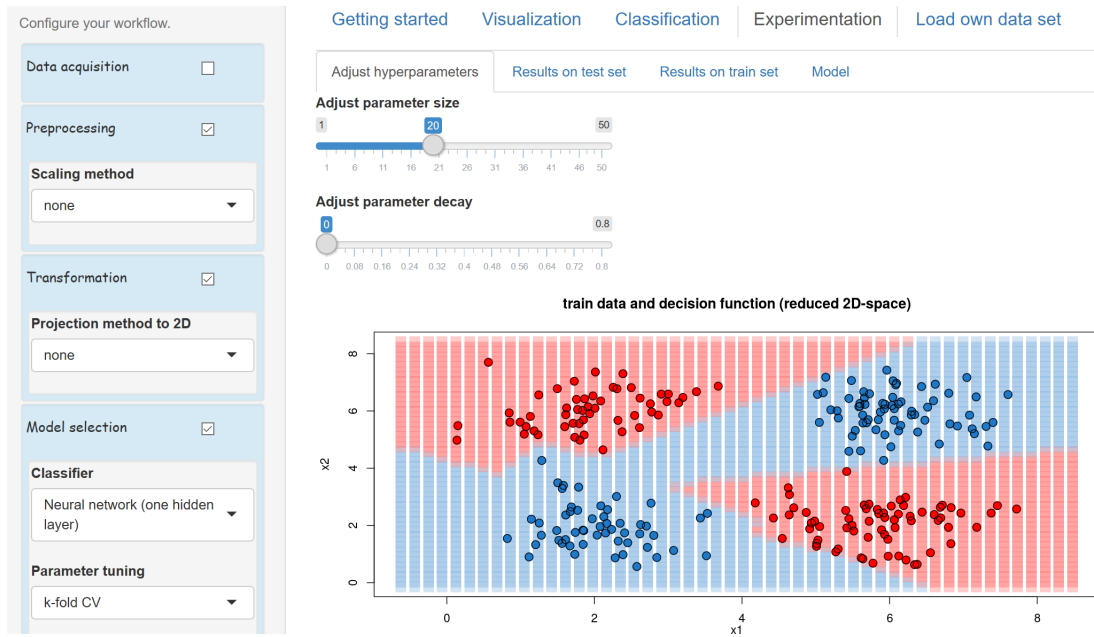
Figure 1. XploreML: In the left pane, the ML pipeline is configured by selecting data sets, attributes, scaling and projection methods and classifiers. The right pane shows visualizations and metrics of the input data ( Visualization ), the classification results ( Classification ), lets the user experiment with hyperparameters ( Experimentation ), allows to upload own data sets and to view and download the extracted executable R source code snippet of the currently configured pipeline.
