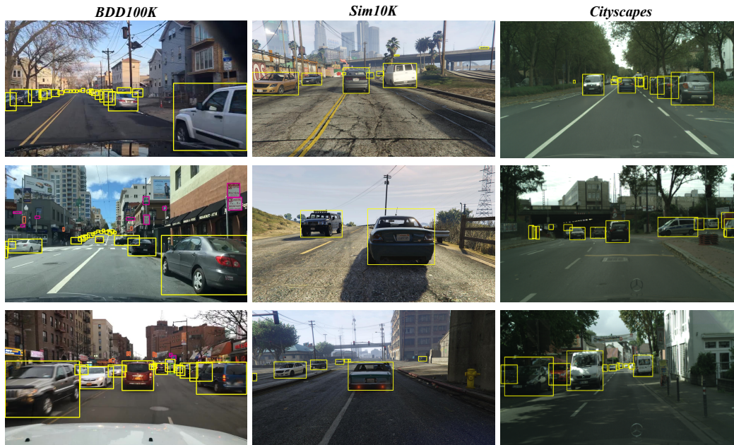
Figure 2: Some samples of datasets included in OOD-ODBench . Note that BDD100K has ten categories while Sim10K and Cityscapes only use the annotated cars.
