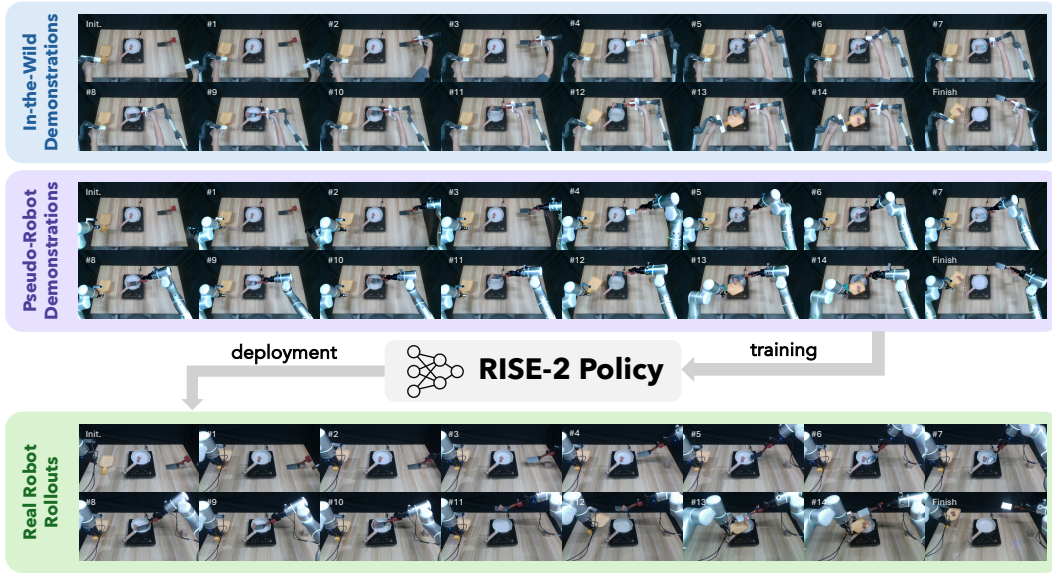
Figure 8: Qualitative Results of the Serve Steak Task. The system is evaluated on a challenging, long-horizon, and contact-rich task, Serve Steak , in which the robot needs to scoop a steak from a pan using a spatula and slide it onto a plate. This task requires precise control across multiple complex steps. We first collect in-the-wild human demonstrations (top) and convert them into pseudo-robot demonstrations (middle) using AirExo-2 . These demonstrations are then used to train the RISE-2 policy, which is successfully deployed on a real robot to complete the task autonomously (bottom).
