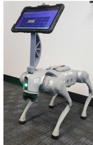
Figure 2: MEMOR-E assistive robot with a head mounted tablet interface used for delivering reminders, cognitive games, and memory oriented interactions.
