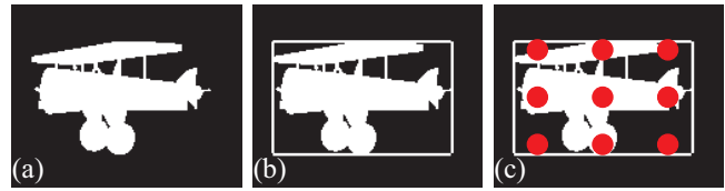
Figure 3: Illustration of shooting rays. We shoot rays within the bounding box of silhouette (b) on image (a) with a subsampling factor in (c).
