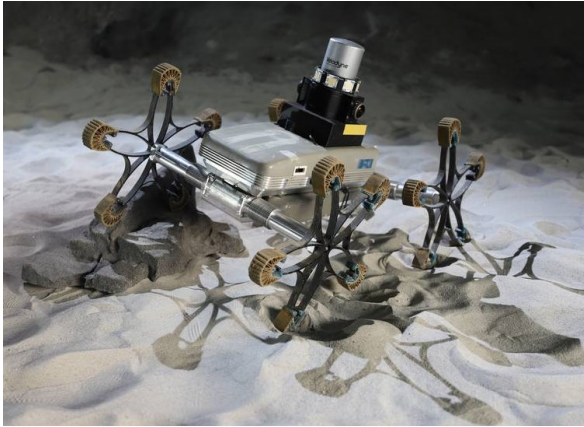
Figure 1. The AsguardIV is a hybrid leg-wheel robot designed at the DFKI to allow navigation in unstructured environments. Its rimless wheels are simpler, more energy-efficient, and more reliable than articulated legs, adapting effectively to obstacles and uneven terrain.
