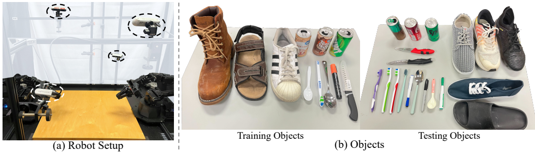
Figure 3: Real Experiment Setup. (a) We use four RealSense cameras to capture RGBD observations and ALOHA robots to execute policy. (b) We test on a diverse set of objects, including shoes, soda cans, marker pens, knives, spoons, toothbrushes, and toothpaste, with diverse geometry and appearance.
