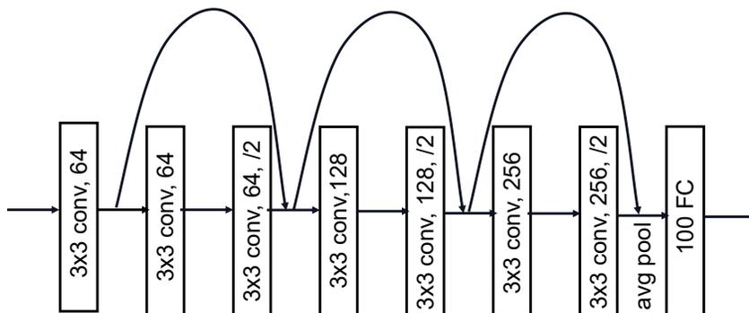
Figure 8: The architecture of ResNet-8.
