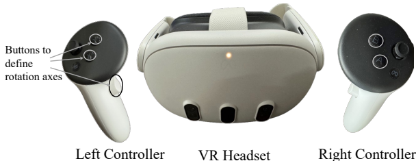
Figure 40: Quest 3 . We teleoperate the arm using the right controller’s pose, while the left controller’s pose specifies the desired rotation axis. We also provide a button-controlled mode that restricts rotation to three fixed axes, selected via the X, Y, and LG buttons on the left controller.
