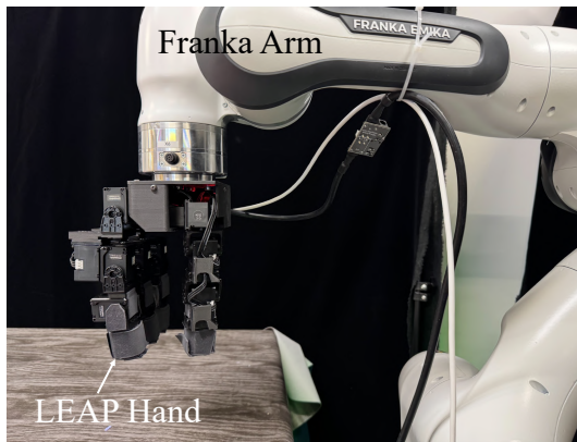
Figure 39: Real World Experiment Hardware Setup.
