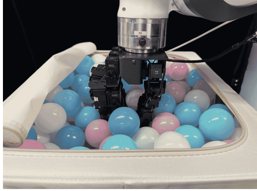
Figure 32: “Half Load” Chaos Box. Instead of totally sinking into balls, the hand only touches the surface of the balls in the box using fingertips.
