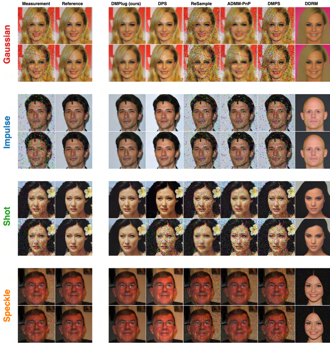
Figure 15: ( Robustness ) Visualization of sample results from the plug-in method ( Ours ) and competing methods for 4\times super-resolution . We generate measurements with four types of noise—Gaussian, impulse, shot, and speckle noise—across two different noise levels: low (level-1) and high (level-2), following [43]. (top: low-level noise; bottom: high-level noise)
