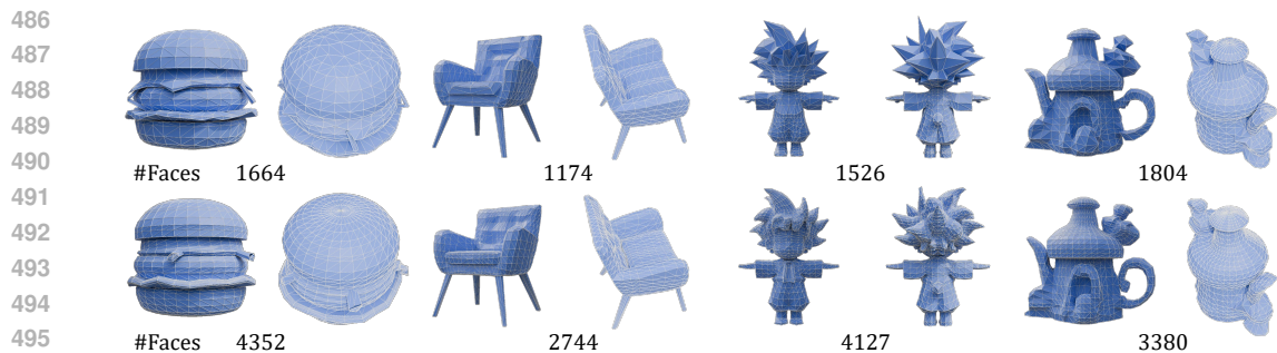
497 Figure 7: Coarse-grained face count control. Our model supports controlling the targeted number 498 of face, which allows to generate meshes with different levels of detail.
