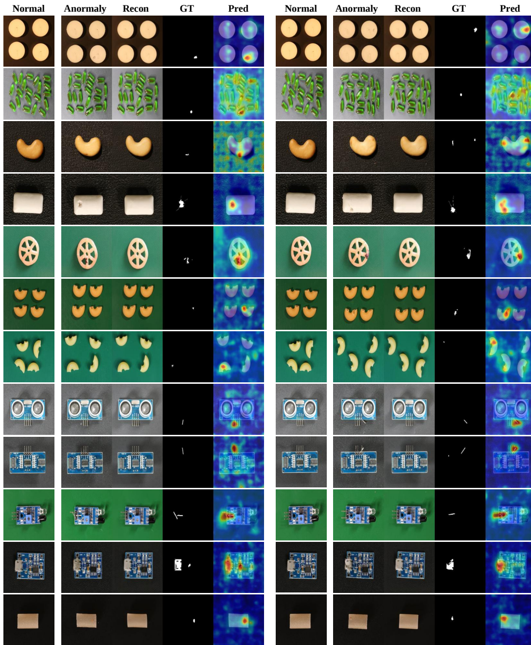
Figure 10. Qualitative results for anomaly localization on VisA. From left to right: normal sample as the reference, anomaly, our reconstruction, ground-truth, and our predicted anomaly map.
