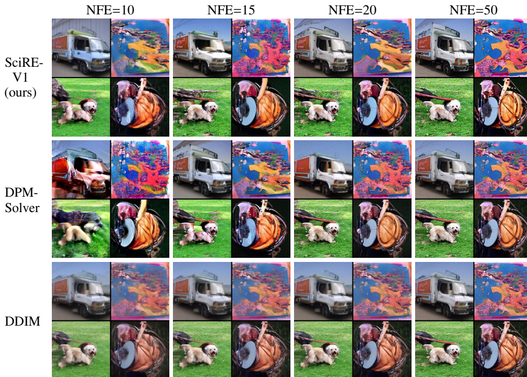
Figure 19: Random samples with the same random seed were generated by DDIM (uniform time steps), DPM-Solver (logSNR time steps), and SciRE-V1 (NSR time steps, k = 3.1 ), employing the pre-trained DPM (Dhariwal & Nichol, 2021) on ImageNet 256 \times 256 (classifier scale: 2.5).
