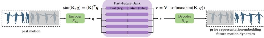
Figure 3: **TransitBank**: Given first half of the motion sequence, it produces a prior representation for the second half of the sequence by computing the weighted average of the values of the bank items to reduce the uncertainty and ambiguity in motion prediction.
