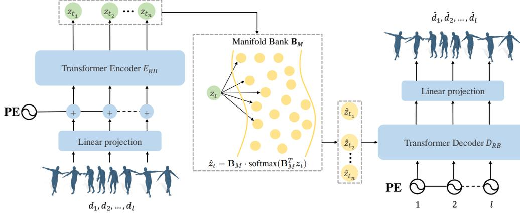
Figure 2: **RefineBank** takes a motion sequence with  $l$  frames as input, projects them to a low-dimensional manifold, and reconstructs the sequence with minimum noise.
