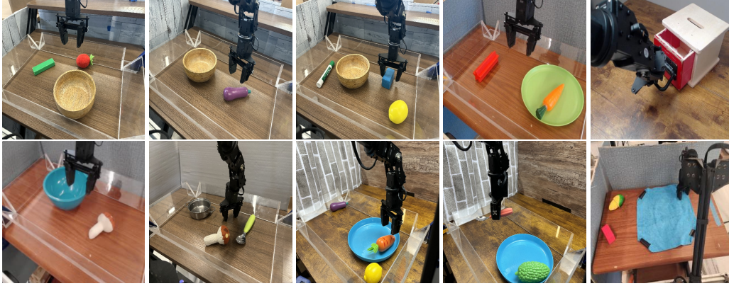
Figure 4: Across the five unique robot workspaces for the five WidowX robots, there are 10 different scenes, each scene corresponding to a distinct set of manipulatable objects available, and each scene supporting many different tasks that can be executed. 8 scenes support pick-and-place tasks, 1 supports drawer opening and closing, and 1 supports deformable cloth manipulation.
