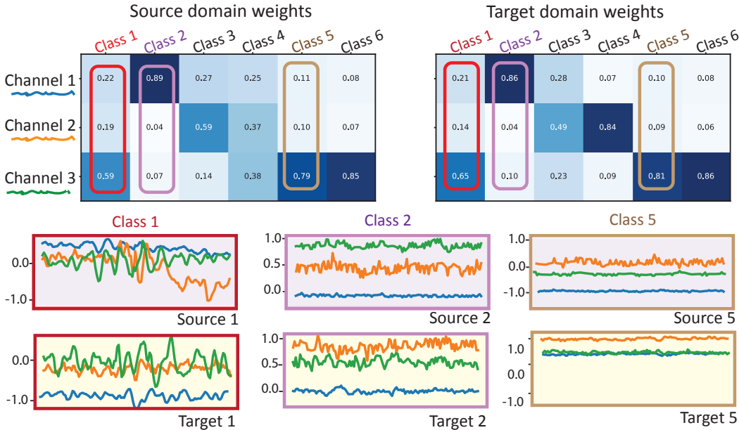
Figure 5: Visualization of channel selection process. The top row shows channel weights learned by our model on the HHAR dataset for the corresponding input data below. The overall weight distribution across the two domains is mostly similar. The colored boxes in the matrices highlight how weights learned for different classes help mask channels with larger shifts between the domains, contributing to improved domain adaptation performance.
