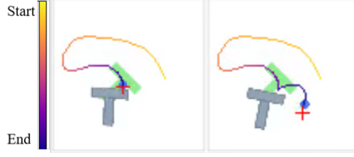
Figure 6: Non-Smooth Trajectory Generation. A Push-T trajectory generated by our Neural SDE, showcasing its ability to handle drastic changes in direction.
