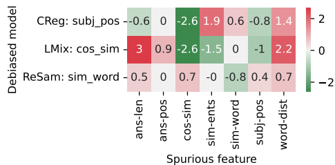
Figure 6: Cross-bias evaluation of debiased models. A relative change of Prediction bias by all spurious correlations, caused by applying inspected debiasing methods on BERT-BASE QA model, in addressing specified spurious correlation. A full matrix is in Appx. A, Fig. 7.
