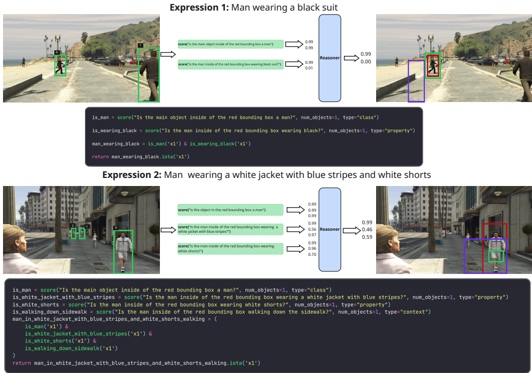
Figure 3: Qualitative examples of NePTune on the RefGTA dataset. Green boxes indicate objects detected by Grounding DINO, blue boxes show objects selected by the VLM (InternVL2.5-8B), and red boxes highlight the final selections made by NePTune.
