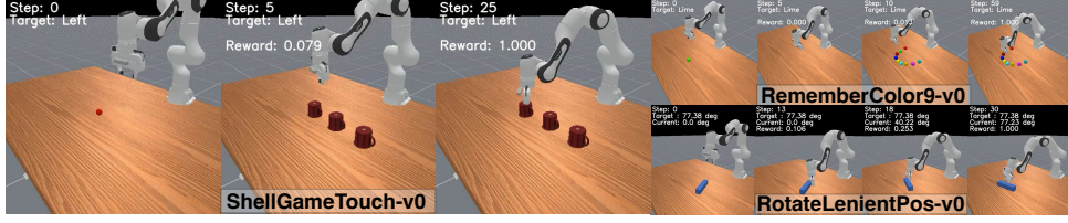
Figure 2: Illustration of demonstrative memory-intensive tasks execution from the proposed MIKASA-Robo benchmark. The ShellGameTouch-v0 task requires the agent to memorize the ball’s location under mugs and touch the correct one. In RememberColor9-v0 , the agent must memorize a cube’s color and later select the matching one. In RotateLenientPos-v0 , the agent must rotate a peg while keeping track of its previous rotations.
