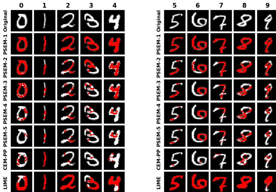
Figure 3: PSEM, CEM-PP, and LIME are demonstrated on digits 0-9 from the MNIST dataset. Red pixels highlight what is sufficient for PSEM along the path, what is sufficient for CEM-PP using the same \beta as in PSEM-3, and what is deemed positively relevant by LIME.
