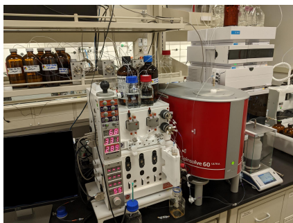
Figure 6: Our laboratory setup for performing the physical experiments. From left to right on the workbench are the lab workstation running the LVCP, the Vaportec CFR unit with automated feed, and the Magritek NMR recording results.
