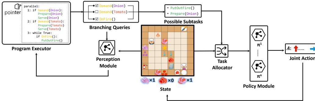
Figure 1: **The overall framework of E-MAPP.** E-MAPP includes four components: 1) A perception module that maps a query  $q$  and the current state  $s$  to boolean responses. 2) A program executor that maintains a pool of possible subtasks and updates them according to the perceptive results. 3) A task allocator that chooses proper subtasks from the subtask pool and assigns those to agents. 4) A policy module that instructs agents in taking actions to accomplish specific subtasks.
