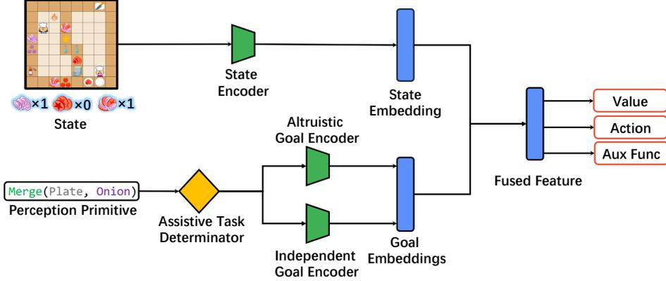
Figure 3: **The policy module.** We adopt a goal-conditioned reinforcement learning framework to determine the policy. We encode goals with a goal encoder and fuse them into the state features. If an agent is assistive, the goal is encoded with an altruistic goal encoder instead. The network has three outputs, including the value function, the action distribution, and the auxiliary functions.
