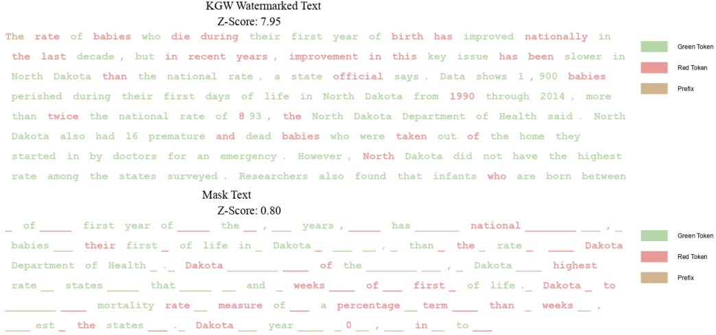
Figure 2: Visualization of watermark text and the text after masking. We can find that according to self-information filter, the mask text significantly reduce the z-score and remove most of the green tokens. Note that actual z-score is lower since some placeholder which will be removed in next step are treated as green token by detector. The shown text are using KGW-1 watermark.
