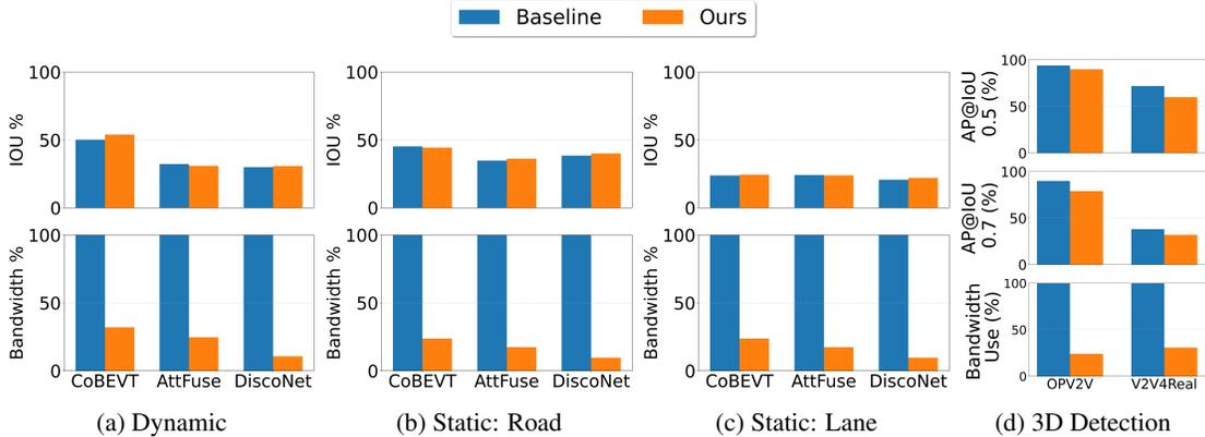
Figure 2: “Trimming” existing cooperative perception baselines, COOPERTRIM reduces bandwidth significantly while preserving accuracy in segmentation (across different semantics, *i.e.*, dynamic, static road, and static lane) and 3D detection tasks.
