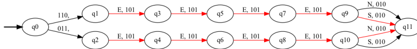
Figure 3: Automaton obtained from T-maze environment with restricted actions. The edges are labelled as [action, observation, reward] .
