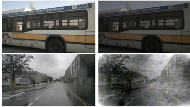
Figure 6: Frequency Jitter at image level. The top line is adjusting the amplitude. It mainly influence the image brightness. The bottom line is adjusting the phase. As it can be, main structures of different targets have been retained.
