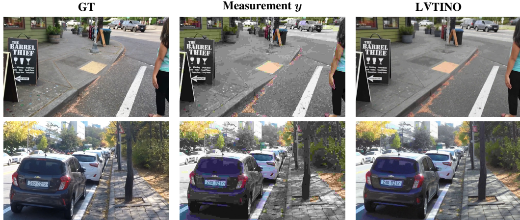
Figure 8: Results on a non-linear inverse problem (Gaussian Noise + JPEG compression). Top row: Example from Adobe240. Bottom row: Example from GoPro240. LVTINO effectively removes blocking artifacts and noise in both cases.
