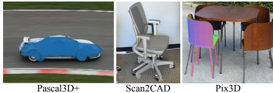
Figure 2: 2D-3D alignments from existing datasets have issues as 3D models do not exactly match the corresponding 2D image due to model discrepancies.
