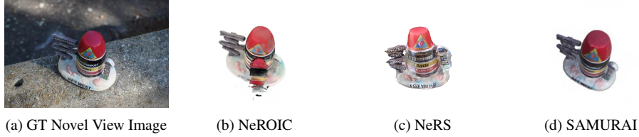
Figure 6: Novel view synthesis with in-the-wild 3D reconstruction. Sample novel view synthesis results of different techniques for 3D reconstruction from in-the-wild image collections.
