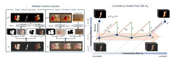
Figure 2: Consistency-Guided Flow SDE  $\Phi_{CF}$ . The masked inversion process (left) combines inverted and noisy latents to obtain the starting latent for optimization. The iterative consistency optimization (right) via consistency-guided flow SDE refines this latent to produce semantically or photorealistically consistency-optimal videos.
