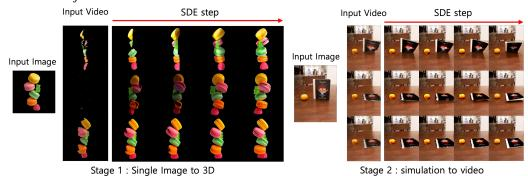
Figure 6: Ablation on the number of Consistency-Guided Flow SDE steps. **Left:** Stage 1 (Single Image to 3D). **Right:** Stage 2 (Simulation to Video). For both stages, the result in the second column (SDE step = 0) corresponds to the result of the standard generation process without SDE optimization.
