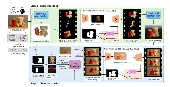
Figure 1: **Overall Pipeline.** Starting from a single image, 3DPHYSVIDEO reconstructs 3D scene geometry via 360-degree orbit video synthesis, then conducts particle-based physics simulation to produce photorealistic videos from the simulation results.
