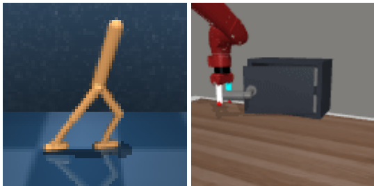
Figure 2: Our image-based environments: The observations are 64 64 and 128 128 raw RGB images for the wal ker-wal k and sawyer-door tasks respectively. The sawyer-door-cl ose environment used in in Section 5.1 also uses the sawyer-door environment.
