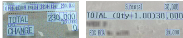
Figure 2: The reading order issue of scanned documents in real-world scenarios. Left: The entity "TOTAL 230,000" is disordered when reading from top to down. The entity "CASH CHANGE" lies in multiple rows and is separated to two segments. Right: The entity "TOTAL 30,000" is interrupted by "(Qty 1.00)" when reading from left to right. All these situations result in disordered model inputs and affect the performance of sequence-labeling based VrD-NER methods. More real-world examples of disordered layouts are displayed in Figure 7 in Appendix.
