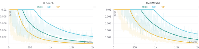
Fig. 10: Training convergence curves. Mean squared error (MSE) loss over training epochs for RLBench and MetaWorld tasks. FDP consistently converges faster and more stably than MoDE and SDP, indicating improved training efficiency and optimization stability.
