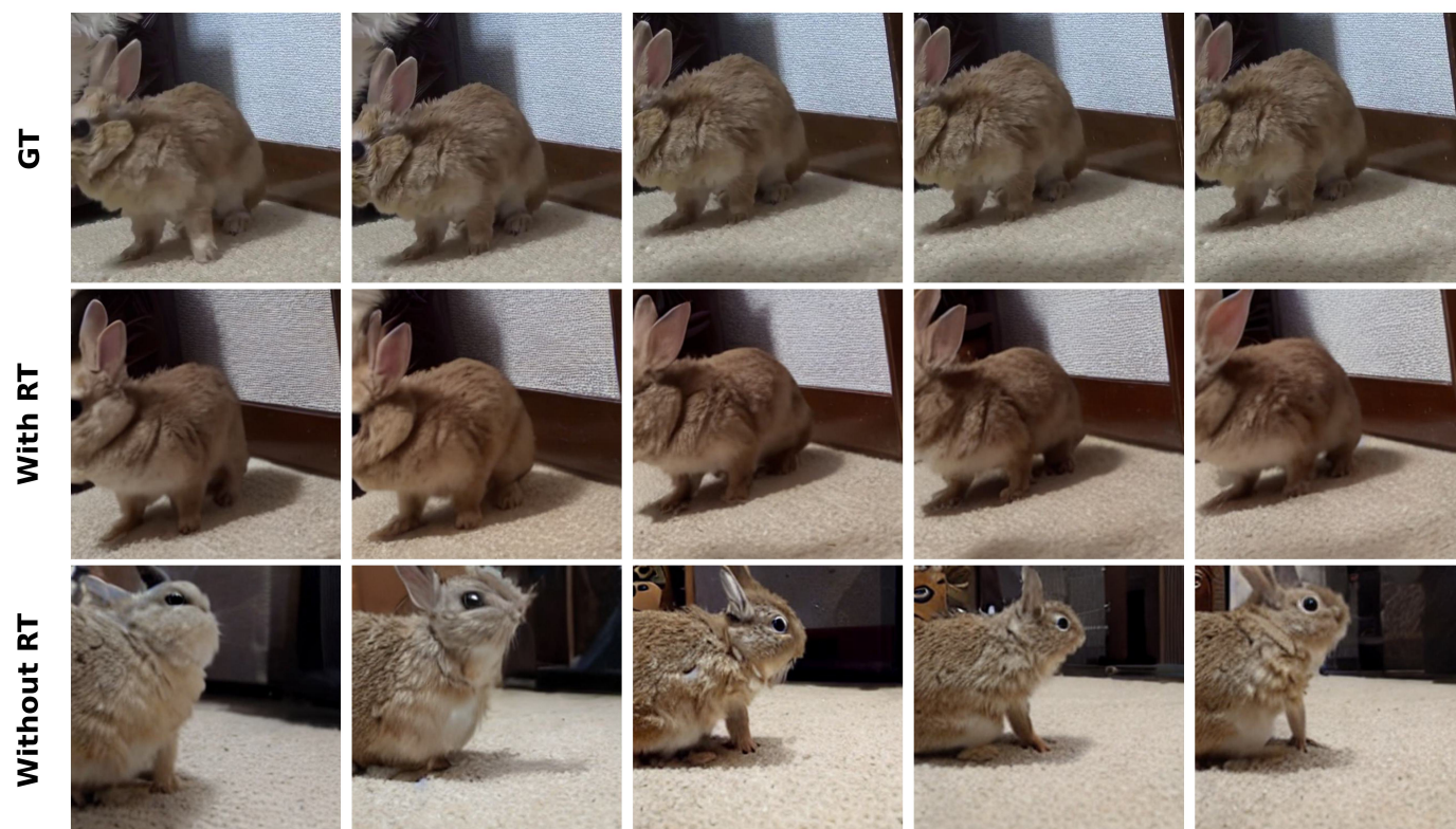
Fig. 14. Temporal video generation results with and without register tokens on YTVIS dataset. Results without register tokens (bottom) lead to spatial inconsistencies across frames. Results with register tokens (middle) maintain consistent object positioning relative to ground truth (top).
