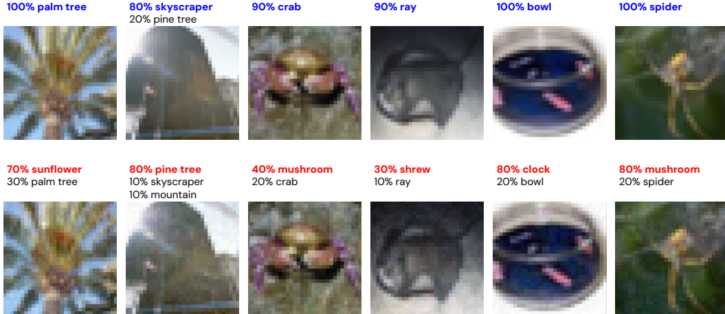
Figure 22: Examples of successfully attacked CIFAR-100 images for an ensemble of self-ensembles – our most robust model. We can see human-plausible ways in which the attack changes the perceived class. For example, the skyscraper has a texture added to it to make it look tree-like.
