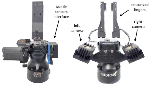
Fig. 2. Mechatronic tool for connector assembly comprising a converging stereo-based camera system and sensorized fingers.
