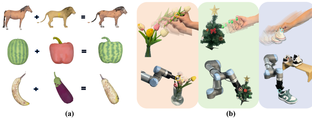
Figure 1: (a) Zero-shot color transfer between 3D assets. (b) In real-world robotic experiments, we use DenseMatcher to transfer a manipulation sequence to the robot from a single human demonstration. Circles represent the contact points in the human demo / grasping points for robot manipulation.
