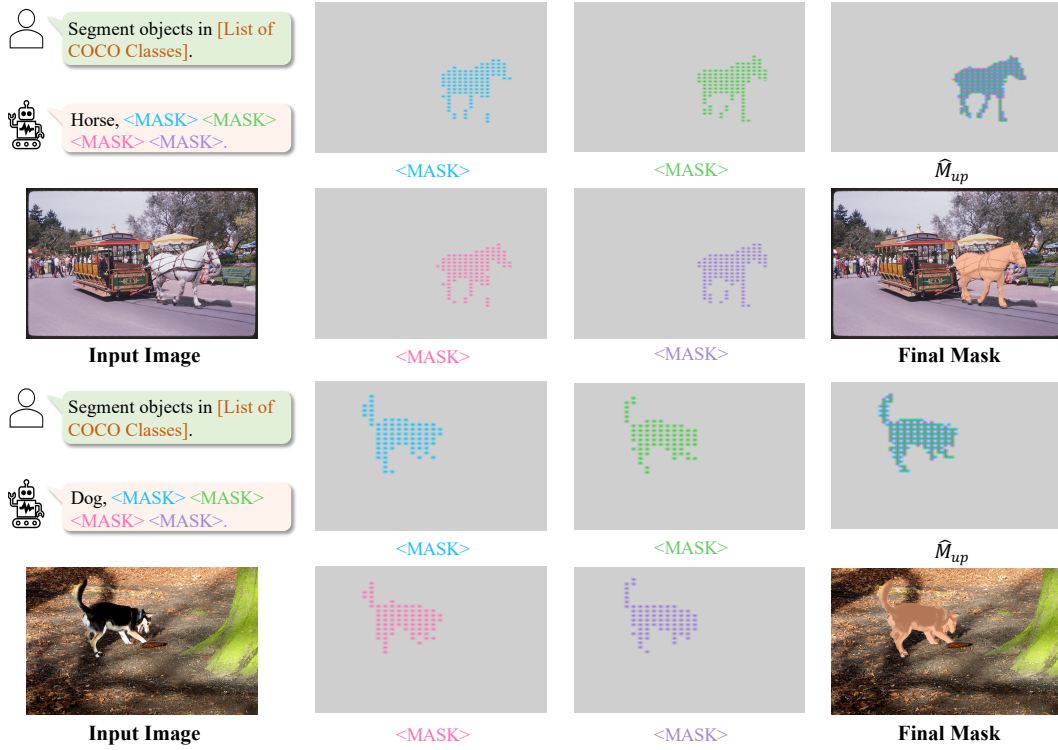
Figure 8: Visualization of multiple mask tokens. We illustrate with four mask tokens (with N=2 ). Employing multiple mask tokens allows for capturing finer details, such as the horse leg and the dog tail, resulting in more precise and refined masks.
