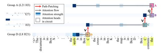
Figure 1: **Entity Tracking circuit in Llama-7B** (*Cir*). The circuit is composed of 4 groups of heads (A,B,C,D) located at the last token (A,B), query label (C), and previous query label (D) token positions. Each group is illustrated by a prominent head in that group.
