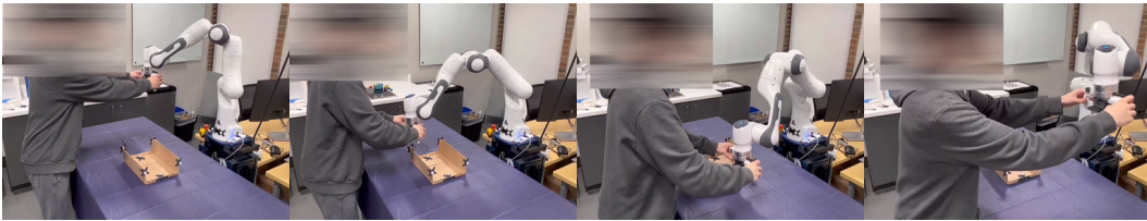
Figure 36: The human guides the end-effector for an inspection task, starting from the left side, passing through a tunnel, and stopping on the right side
