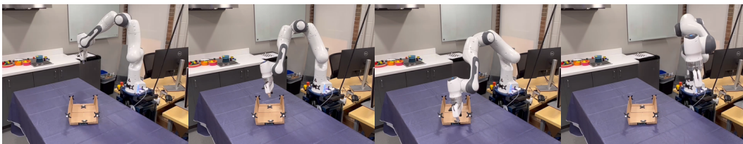
Figure 38: The tunnel is rotated. We rotate the end-effector to be parallel with the tunnel before the execution.
