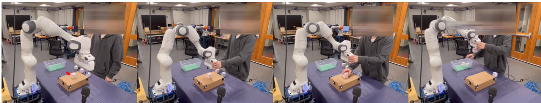
Figure 35: The cube was shifted slightly to the right side of the robot (The shifting direction is indicated by the red arrow). During the execution, the human held the robot and switched to another cube. After that, the robot finished the task
