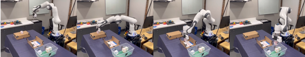
Figure 41: Composing the learned DSs with task transfer parameters from the “pick and place” and “tunnel” tasks. The robot is able to pick up a block, pass through the tunnel for scanning, and place the block in the bin. The entire motion does not require extra demonstration. Note the positions of the objects are not the same as in the original demonstrations.
