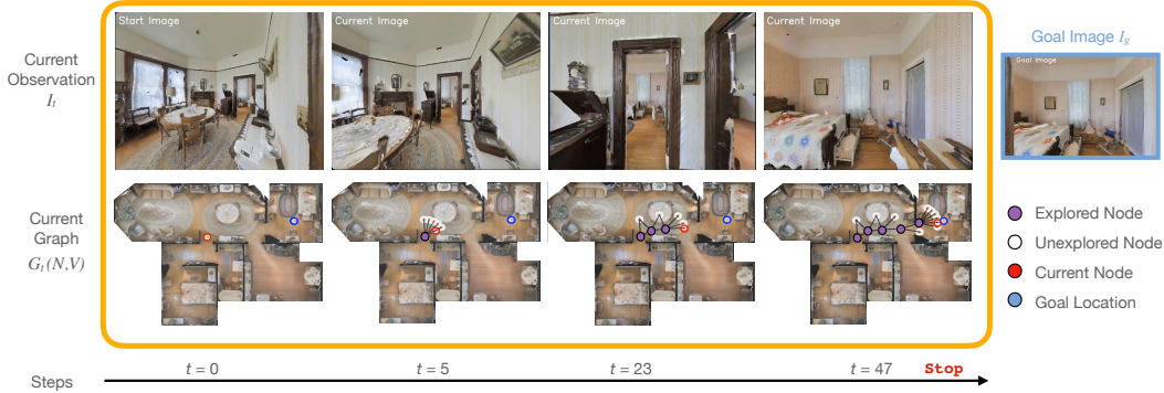
Figure 6: Example of an Image-Goal Navigation episode on MP3D. Shows the agent’s observations and internal topological graph at different time steps.
