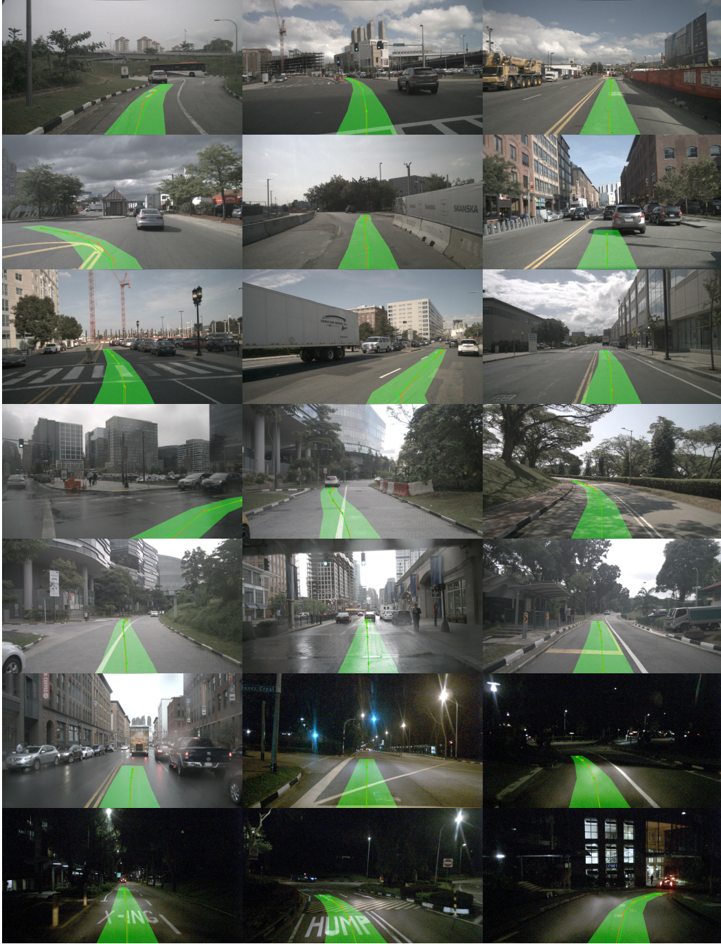
Figure 7: We uniformly sampled more frames from the nuScenes and visualized them. These results are generated using one of the top-performing model checkpoints, with predicted trajectories in green and ground truth in orange.
