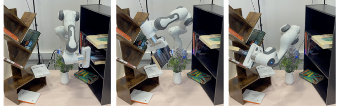
(b) Our policy has not been trained on this bookcase, yet it is able to insert the book into the correct location.
