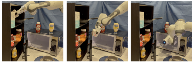
(a) Sampling-based planners struggle with tight spaces, a regime in which Neural MP performs well.
