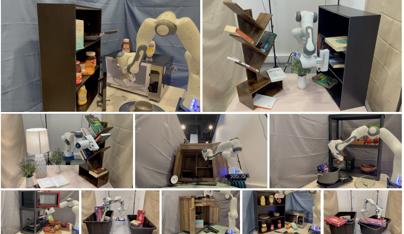
Fig. 1: Neural Motion Planning at Scale in the Real World Our approach enables a single, generalist neural network policy to solve motion planning problems across diverse setups; Neural MP can generate collision free motions for a wide array of unseen tasks significantly faster and with higher success than traditional as well as learning-based motion planning approaches.
