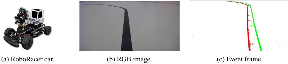
Figure 7: (a) RoboRacer car equipped with Sony/Prophesee IMX636 sensor for the real-world deployment of the proposed algorithm. (b) RGB frame and the corresponding (c) DVS event frame representation.
